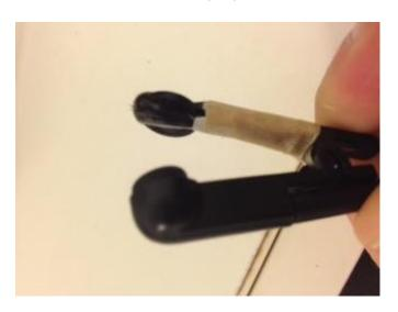
6. The carbon fibres will stick out a bit beyond the auricular clip: take a small strip of masking tape and carefully tape the fibres to the back of the auricular clip.
