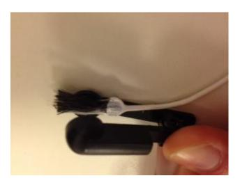
5. Wrap the masking tape around the electrode lead to secure it to the auricular clip. Make sure that the carbon fibres are fully exposed.
